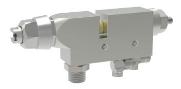
The automatic-spray valve S 830 is an airless spray valve. All connections are mounted on the under-side of valve. The control of valve is reached through two separate air connections. One for the opening of needle and one for the closing of needle. This has to be done via external pneumatic valves.
