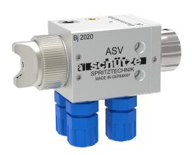
The spray valves of series ASV are pneumatically controlled spray valves. They are suitable for spraying release agents, oils, colours and in version KLS also for glues and adhesives.
