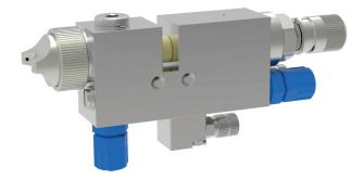
The MKD-IS/ES spray valve is a pneumatically controlled applicator for processing spray materials, e.g. release agents, adhesives or paints. It is suitable for both continuous and intermittent application.
