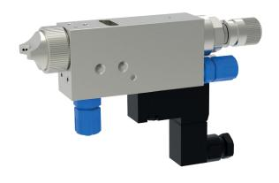
The spray valves of series MKD-IS R/F are electropneumatically controlled spray valves. They are suitable for spraying release agents, oils, colours and in version KLS also for glues and adhesives. The control of valve is done via the direct mounted solenoid valve. The supply of fluid is done via pressure tanks or pumps.
