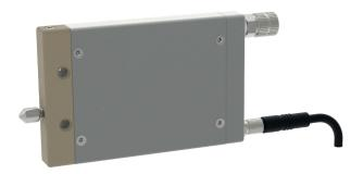
The EMVV electrical full jet valve is an electronically controlled applicator for the processing of materials such as sealants, adhesives, greases, paints, oils and many other media. The spraying process can be carried out as either an intermittent or continuous process.
