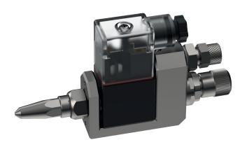
The EVV-2 electric full jet valve is an electromagnetically controlled applicator for the processing of materials, such as sealants, adhesives, greases, paints, oils and many other media. The spraying process can be carried out as either an intermittent or continuous process.
