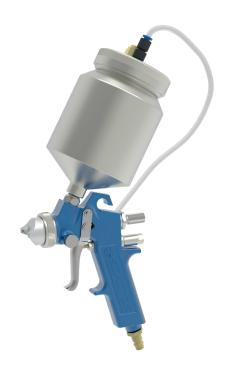
The pressure feed cup spraygun W 4 is equipped with a 0.7 ltr. pressure feed cup. Therefore it's particulary suitable for apply evenly viscous fluids. The pressure of feed cup is alterable by a regulating knob. In this way the quantity of fluid is adjustable to the desired sprayjet.
