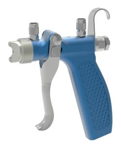
The SCHÜTZE FINE-SPRAY gun W3 FZ-Duo is designed especially to handle sprayable fluids of very low viscosities. Fine co-ordination of precision made nozzle, needle and air cap produce an atomizing result which particularly when applying release agents gives an extreme smooth lay on in moulds and dies.
